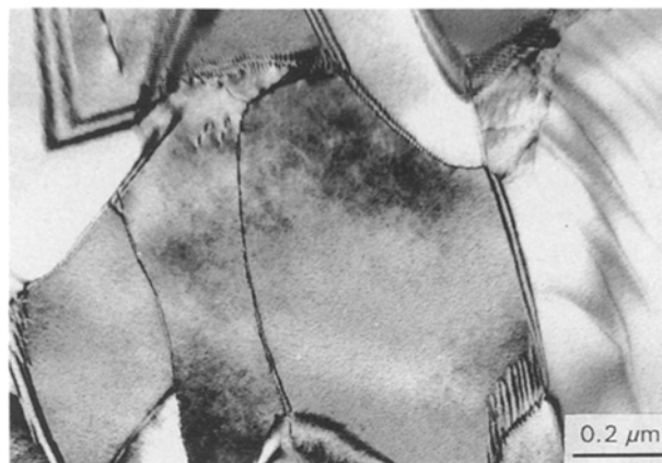
Figure 10 Microstructure of the Al-4% Mg-1% Sc alloy cold-rolled 83% prior to ageing to peak hardness at 593 K (320°C).
